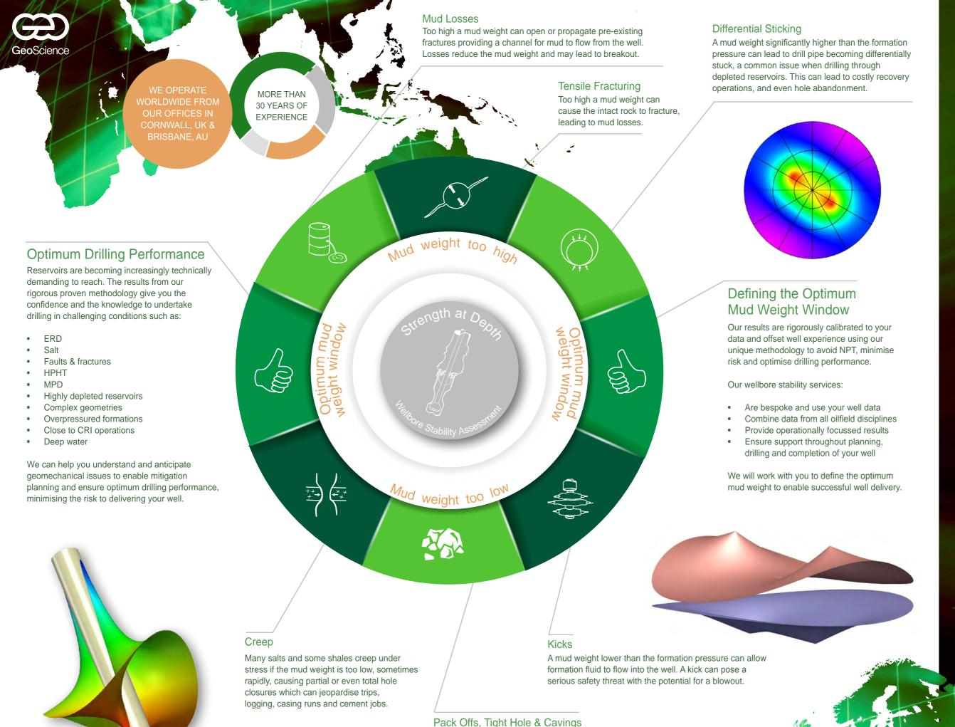
Too low a mud weight can result in cavings as breakout
